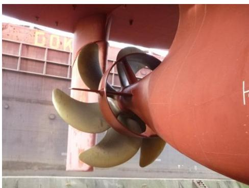
**Figure 2.** Becker Twisted Fin<sup>®</sup>, first installation on a 7090 TEU Container Vessel, Hamburg Süd
