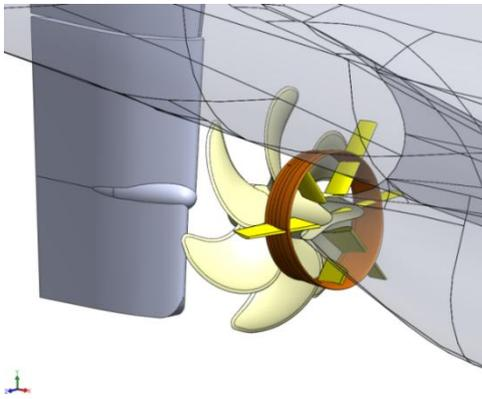
**Figure 1.** Becker Twisted Fin<sup>®</sup> designed for a large container vessel
